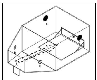
**FIGURE 1.** Disinfection chamber. The dotted arrow represents the direction of disinfectant (or control) flow, following introduction through the A port. Additional airflow was introduced through B ports to provide turbulent mixing of the disinfectant plume. C ports were filtered vents.
